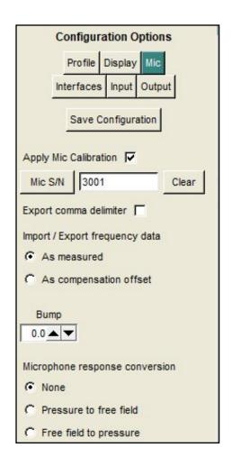
Enable and load microphone calibration file.
